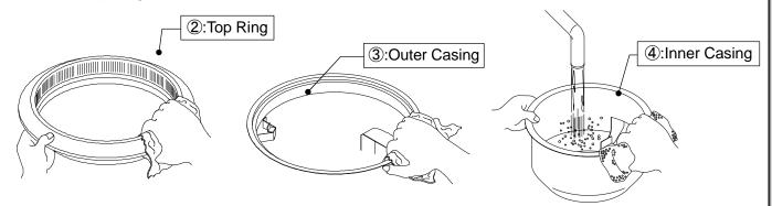
3 Clean the Outer Casing at the close of business. (Remove the Filter Set from the Outer Casing)
