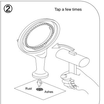
Tap the Burner Head a few times with a plastic or wooden hammer to remove the rust and ashes.
